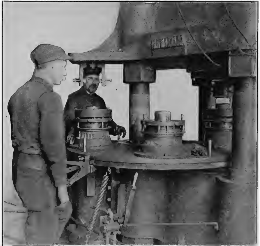
FIG. 5. HYDRAULIC HEADING PRESS FOR 4.5 CARTRIDGE CASES
